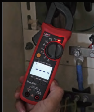
NCV multi-segment display and audio/visual alarm
